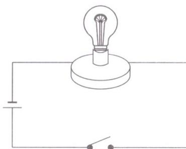
The bulb glows on when the circuit is closed or the switch is switched ON
