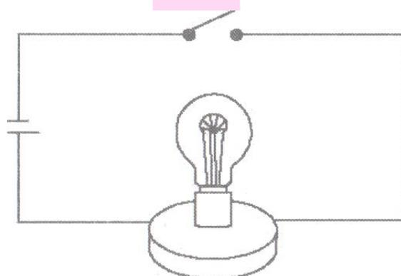
A circuit diagram showing open circuit.
