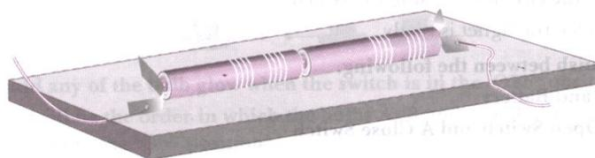
One of the reasons may be that the rubber band used in the cell holder may not be tight enough to keep the two cells in contact with each other. If the cells are not in proper contact with each other, then the circuit will not be complete and current will not flow through the circuit. Hence, the bulb will not glow. The other reason may be that the two cells are not connected properly. The negative terminal of one cell must be connected to the positive terminal of the other cell.
