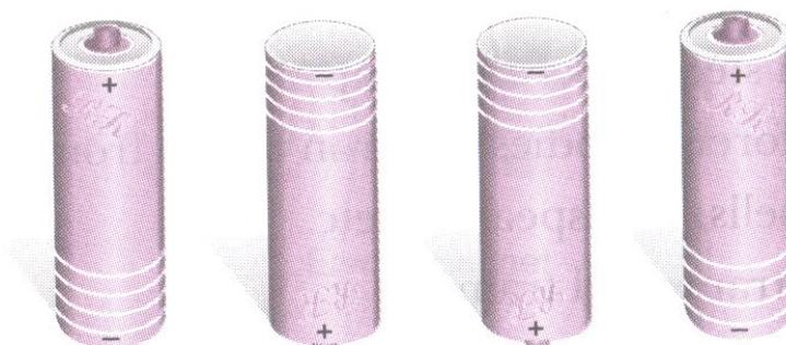
To make a battery, the negative terminal of one cell must be connected to the positive terminal of the next cell with the help of connecting wires.
