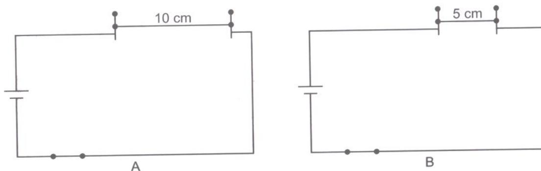
(a) No the amount of heat produced in both the cases will not be equal. Amount of heat produced in a wire depends upon the length of the wire.
