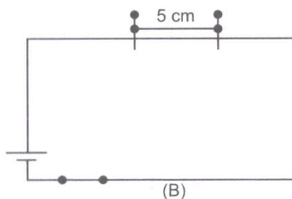
i. No, the amount of heat produced in both the cases will not be equal. Amount of heat produced in a wire depends upon the length of the wire.
