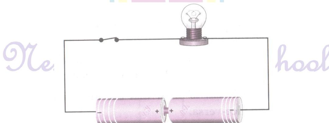
The bulb in the circuit is not glowing because the two cells are not connected properly. To make the bulb glow, the negative terminal of one cell should be connected to the positive terminal of the other cell, as shown in the given figure
